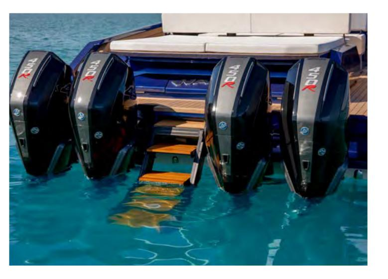
Wally has ingeniously split the four engines to the flanks of the boat, with two on each side, allowing the installation of the retractable hydraulic boarding passerelle/swim ladder to provide direct and easy access to the water or the shore.
